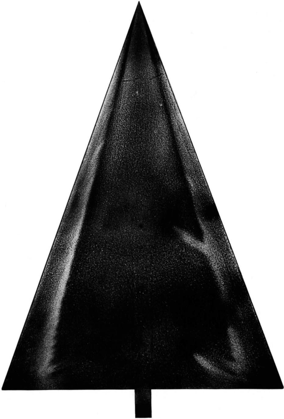
FIG. 35b. 70° delta wing, flat upper surface. Transition pattern at \alpha = 25^\circ .
