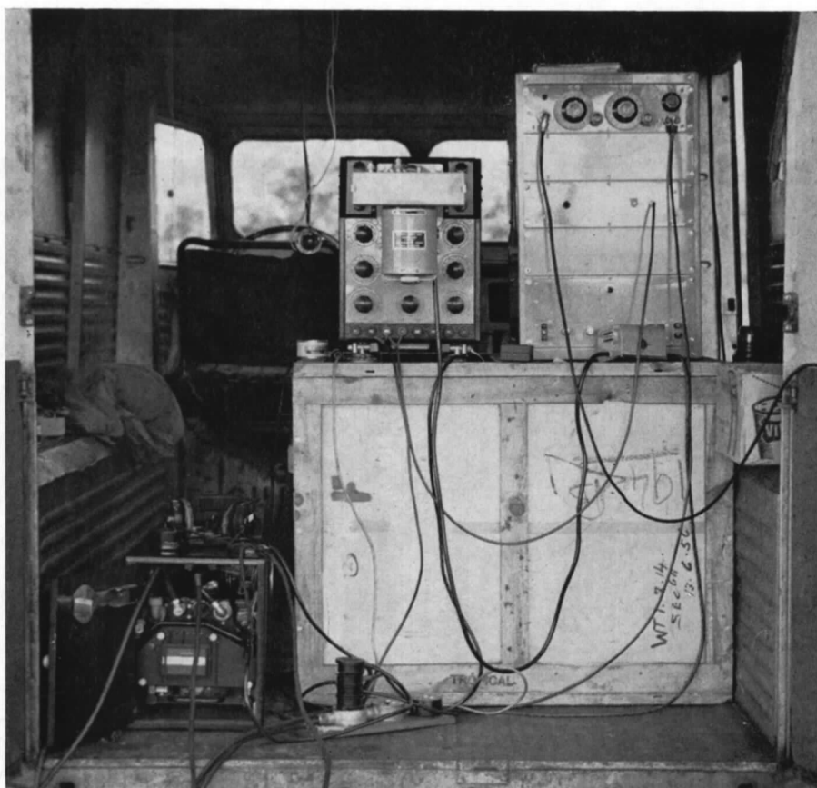
FIG. 3b. Installation of F.M. equipment, recording oscillograph, and intersite communications transceiver in Citroën van at 'Radar' site.
