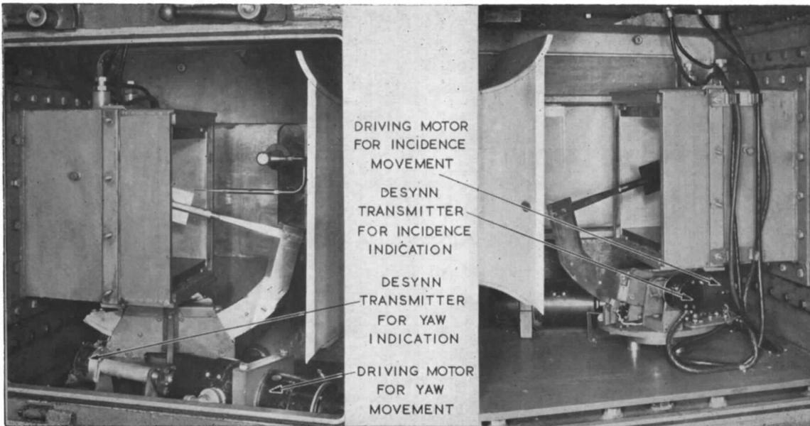
FIG. 2. Model installation in No. 8 (10 in. × 9 in.) Supersonic Tunnel.
