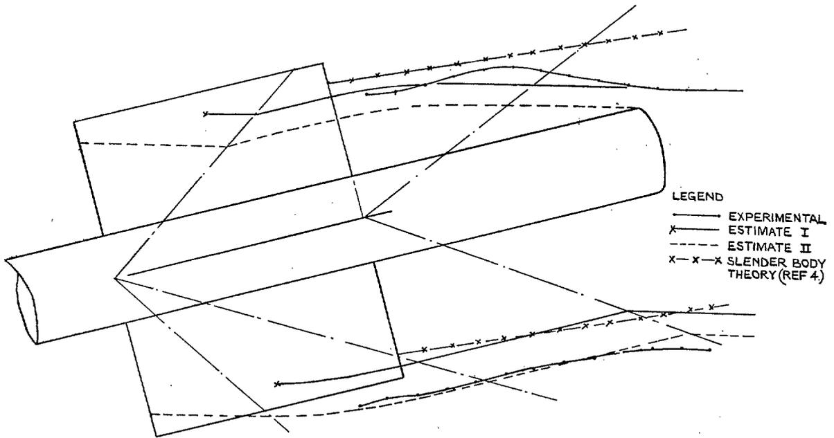
FIG. 25. Vortex-core paths—comparison of estimates with experimental results.
