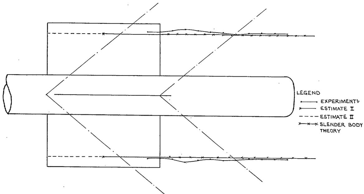
FIG. 22. Vortex-core paths—comparison of estimates with experimental results.
