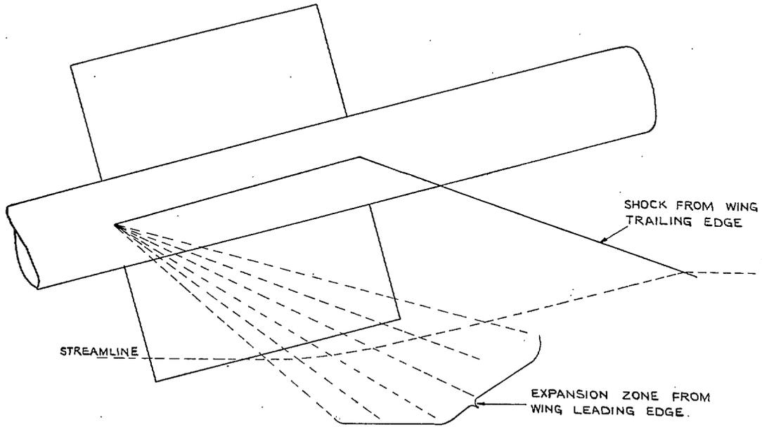
FIG. 21. Sketch showing method of tracing streamline.
