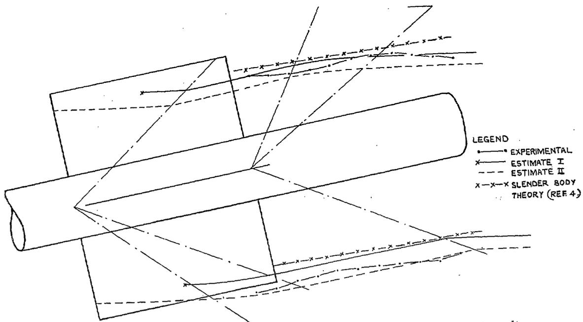
FIG. 24. Vortex-core paths—comparison of estimates with experimental results.
