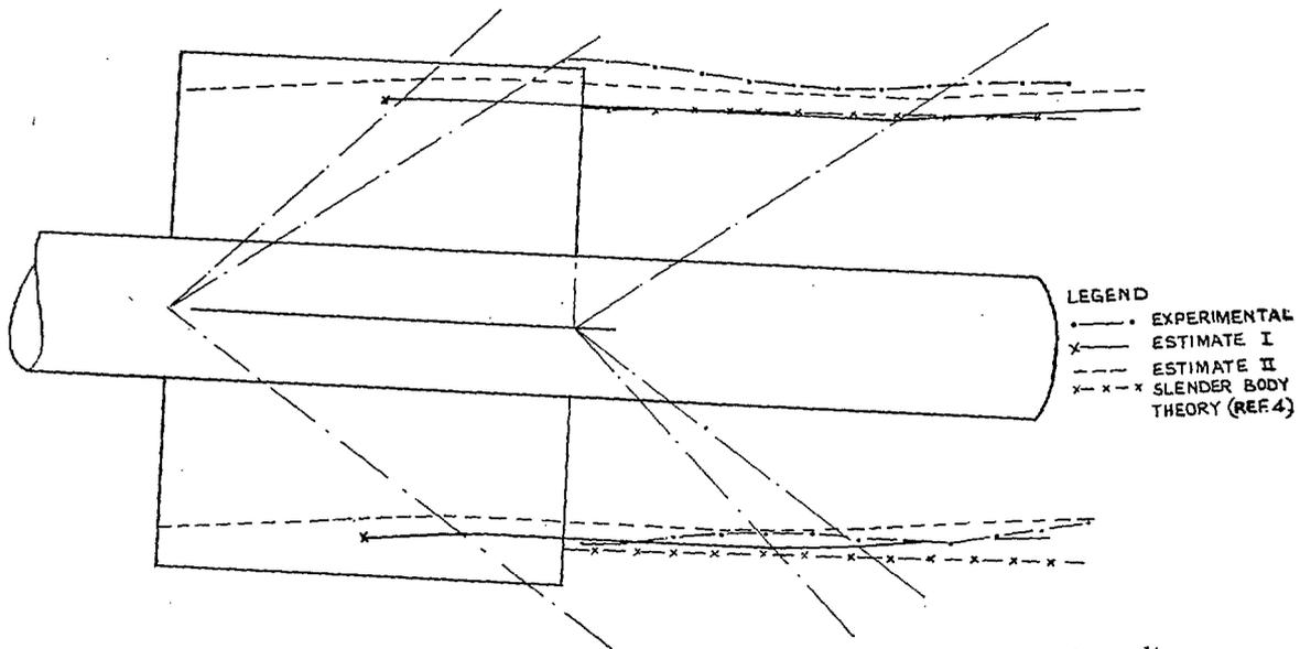
FIG. 23. Vortex-core paths—comparison of estimates with experimental results.
