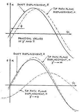
FIG. 3. Attitude *versus* time curves of rotor shaft and tip-path plane axis in steady harmonic motion.
