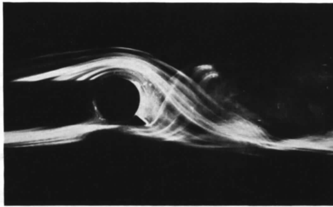
(c) Photograph of the trailing vorticity with flap deflected about 40 deg (off-centre position, side nearest camera).
