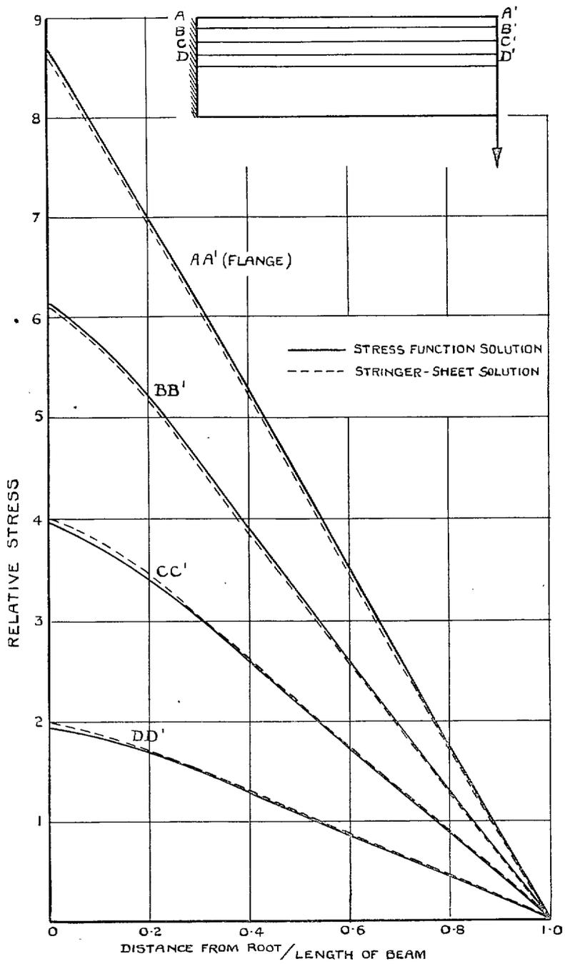
FIG. 3. Longitudinal Stress in Beam of Fig. 1 Subject to Single Transverse Load at Tip
