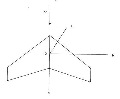
Let V be the velocity of the airstream and let u, v, w be the velocity components of the disturbed flow corresponding to small oscillations or displacements of the flexible surface. Euler's equations for incompressible inviscid flow then gives
