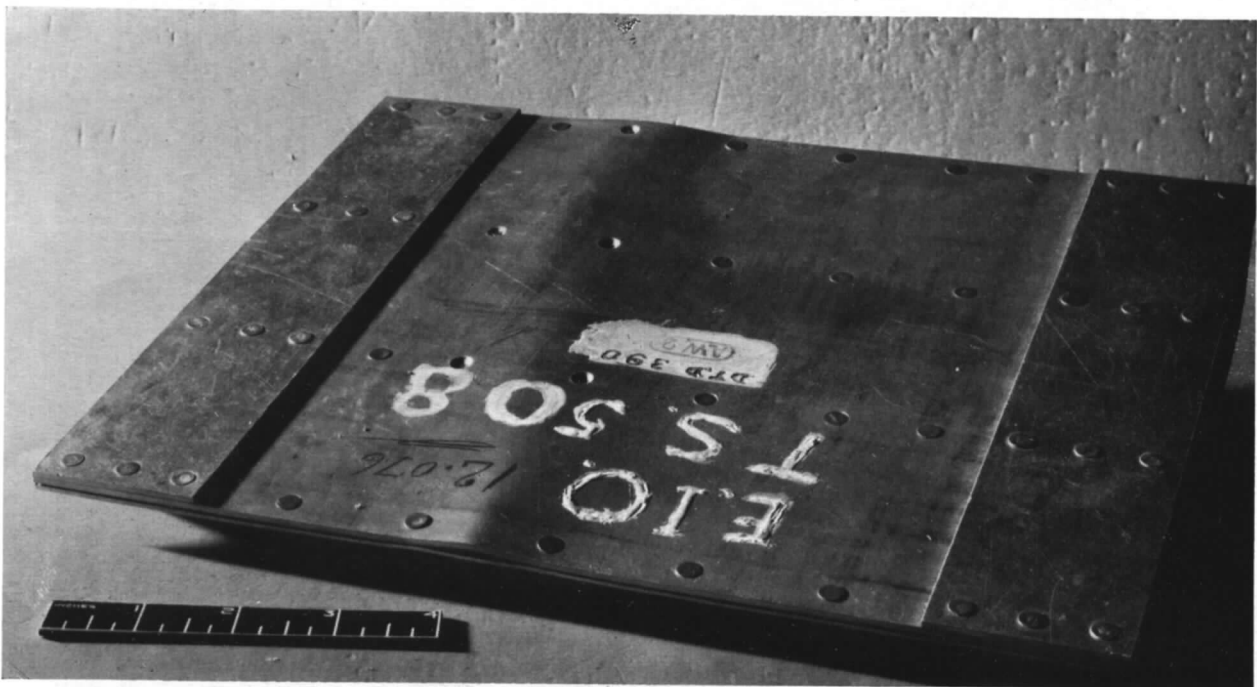
FIG. 28. Specimen Number E10 showing typical diagonal inter-rivet failure for staggered rivets.
