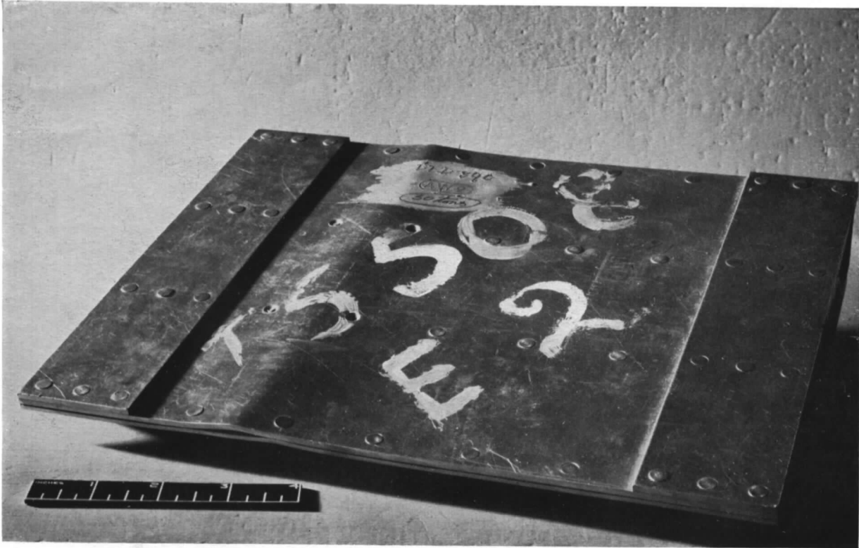
FIG. 27. Specimen Number E2 showing typical inter-rivet failure for unstaggered rivets.
