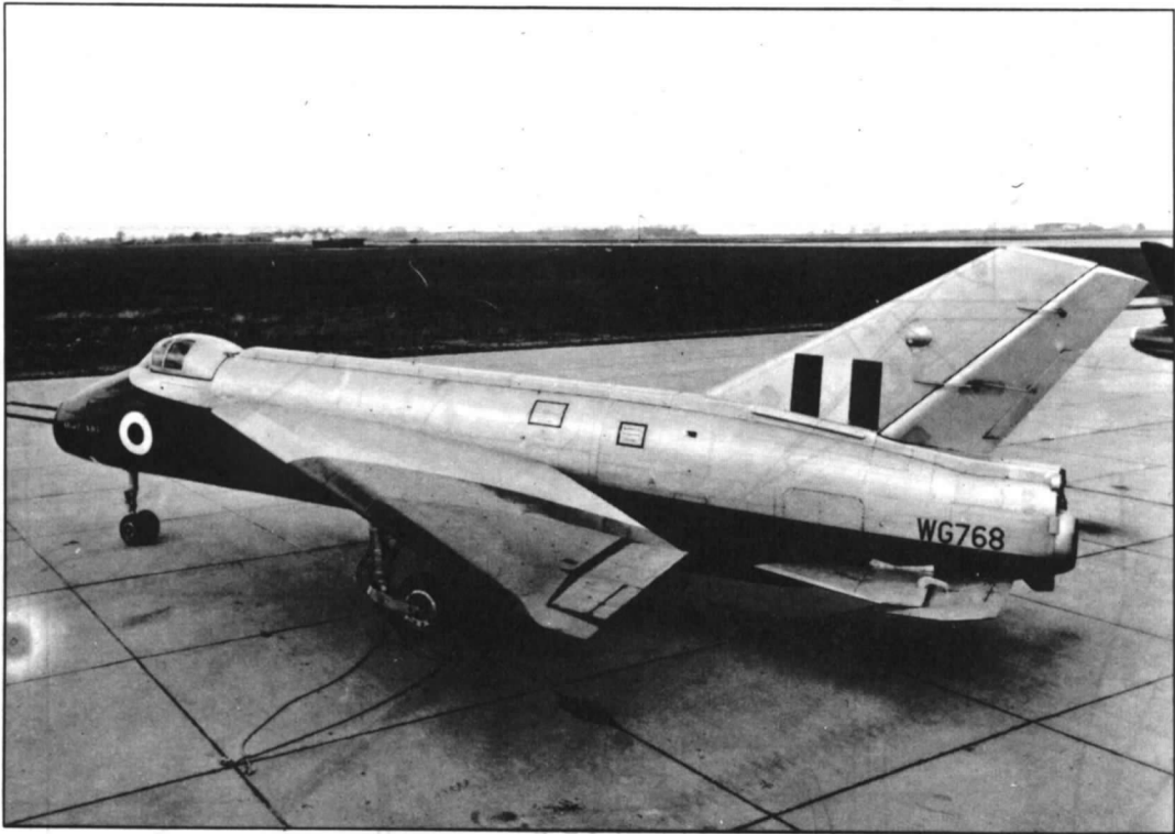
(b) 10.7° full span leading edge droop configuration.
