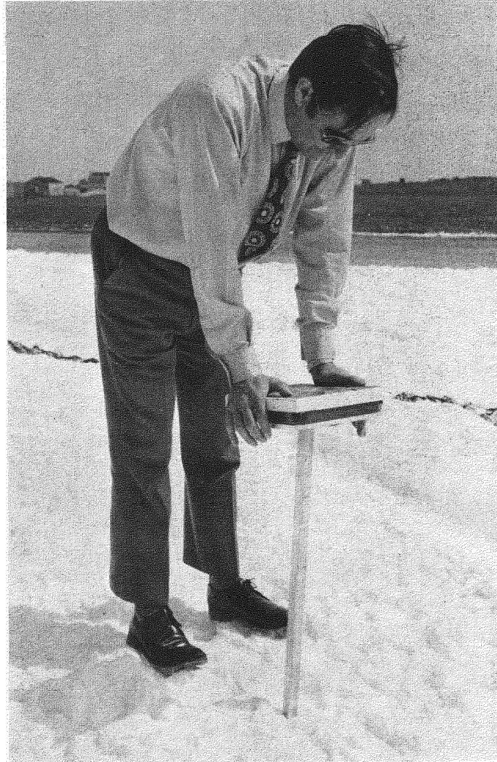
Fig.9 Method employed to measure mean foam crushing strength values
