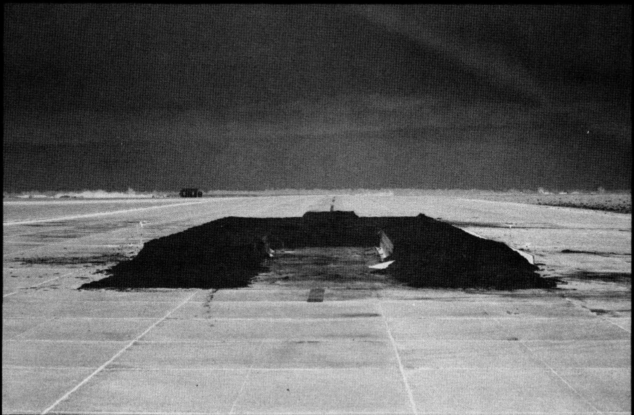
Fig.6 Arrangement of the double layered UF foam test beds used for trials
