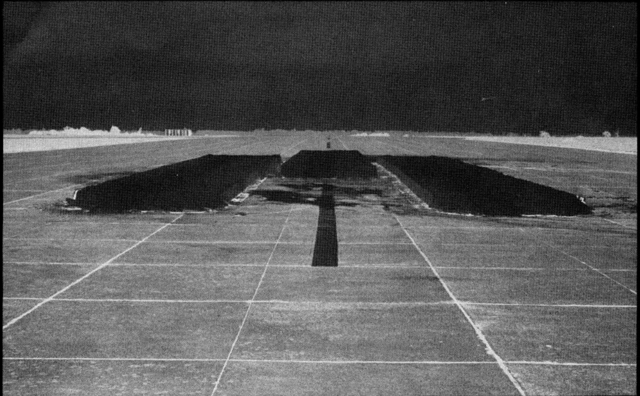
Fig.5 Arrangement of the single layered UF foam test beds used for trials
