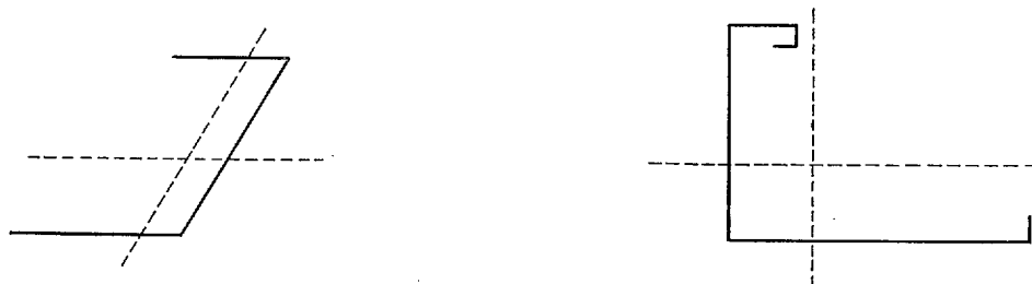
Convenient axes (through centroid) shown dotted.
