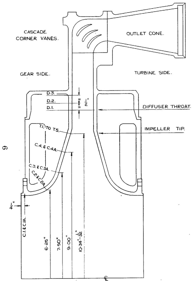
FIG. 3. Location of static points on blower casing.
