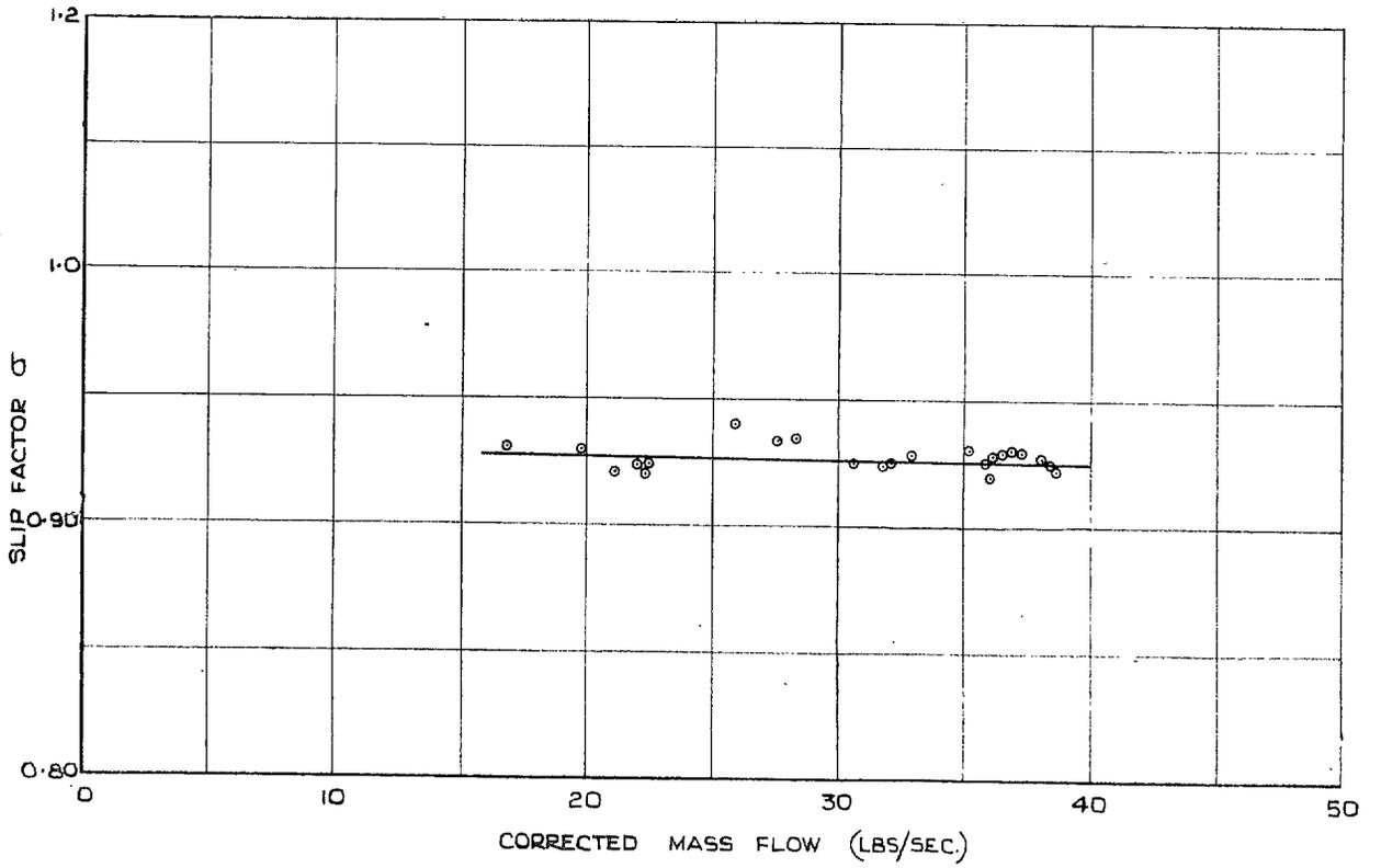
FIG. 10. Slip factor *vs.* corrected mass flow.
