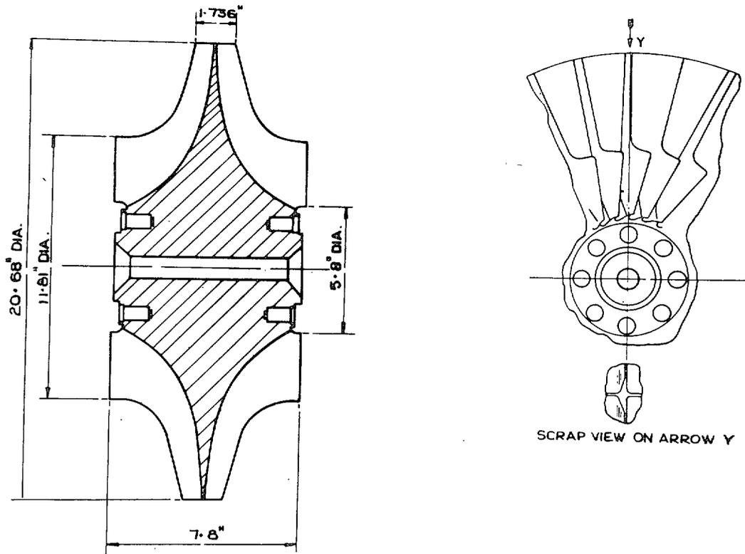
FIG. 1. The No. 8 Design impeller.
