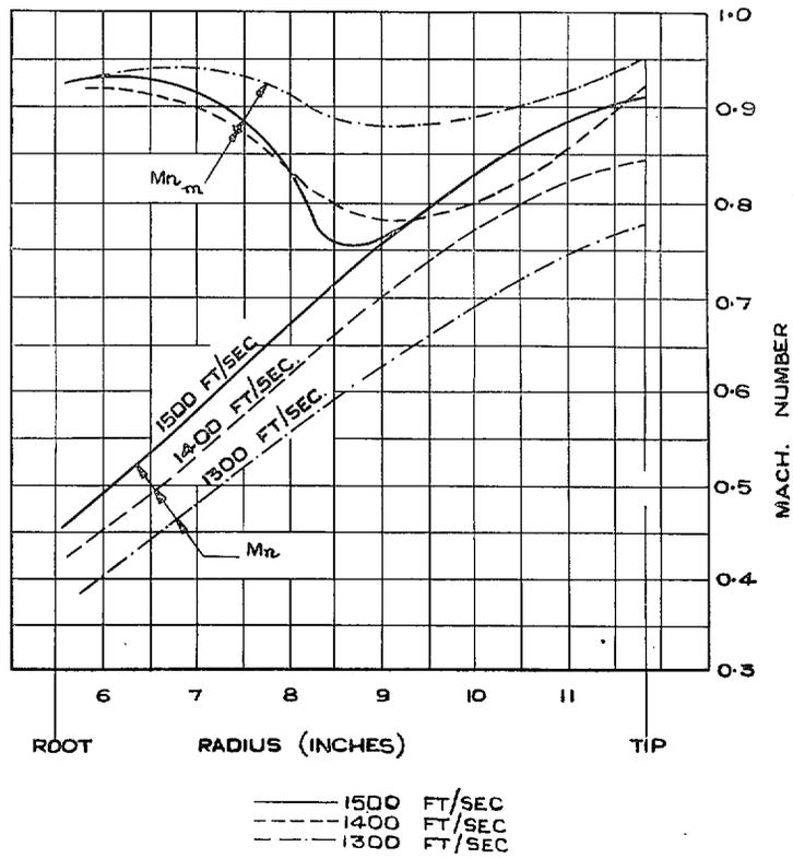
FIG. 7. Variation of Mach number across impeller eye. Choking occurs when  $M_n > M_{n,m}$ .
