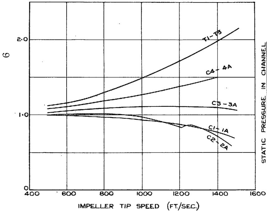
FIG. 8. Static pressures in impeller channels (at peak compression ratio).
