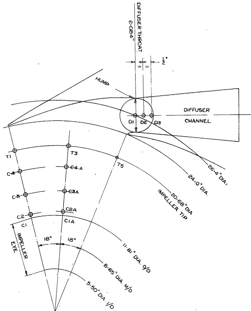
FIG. 4. Location of static points on blower casing.
