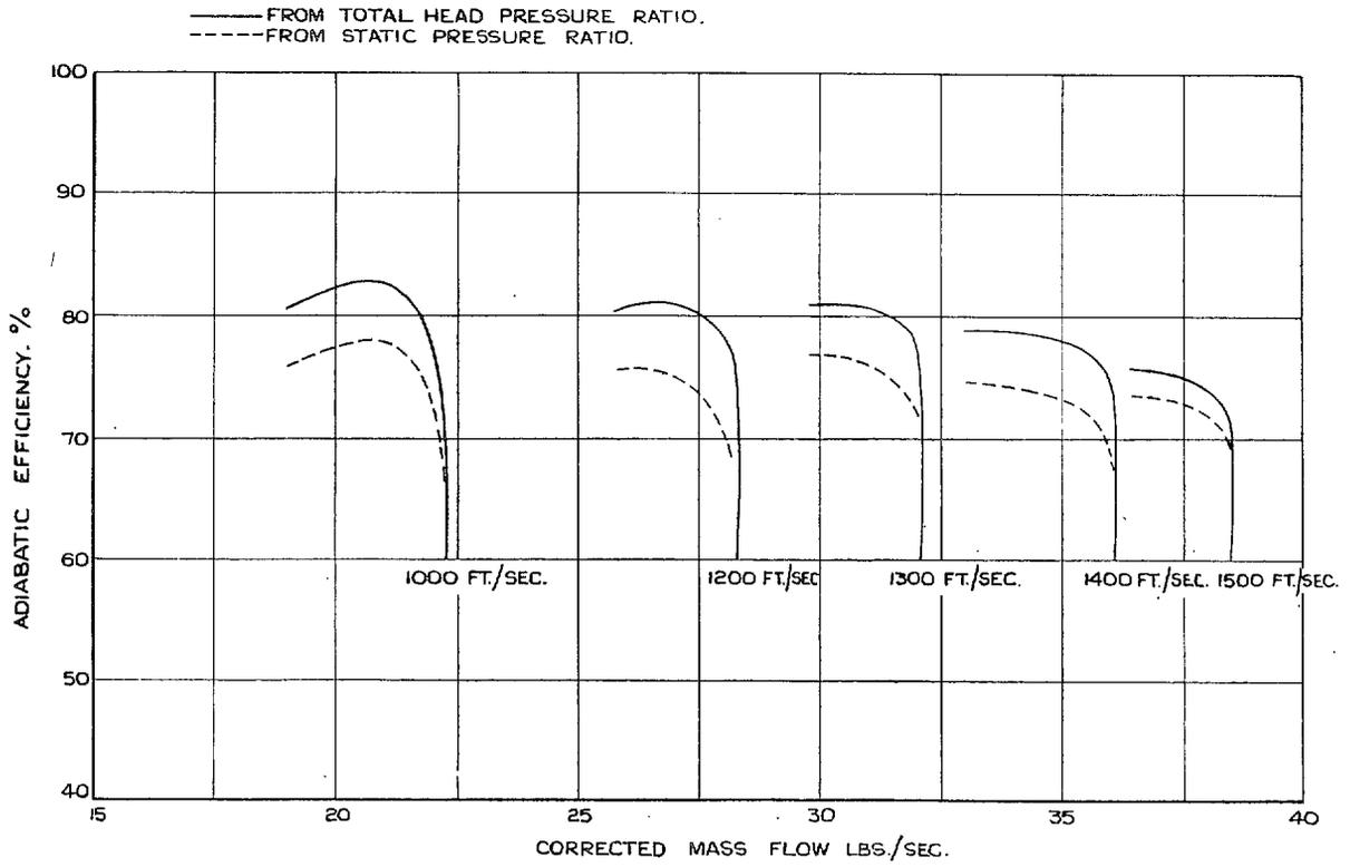
FIG. 6. Overall adiabatic efficiency vs. corrected mass flow.
