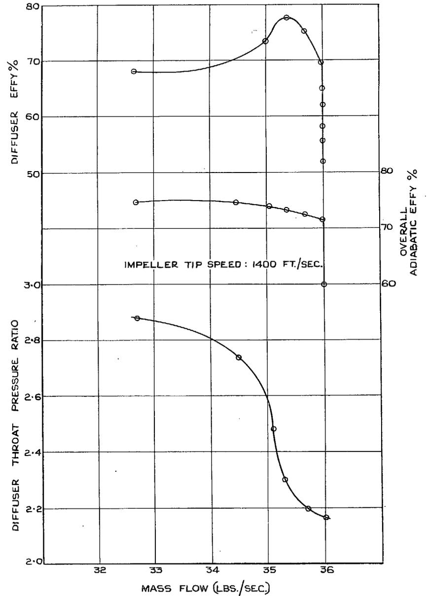
FIG. 9. Diffuser efficiency vs. corrected mass flow.
