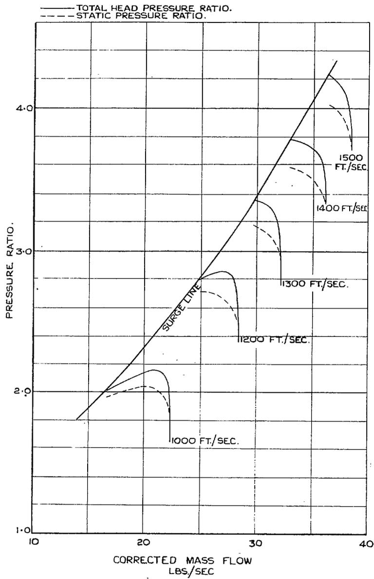
FIG. 5. Pressure ratio vs. corrected mass flow.
