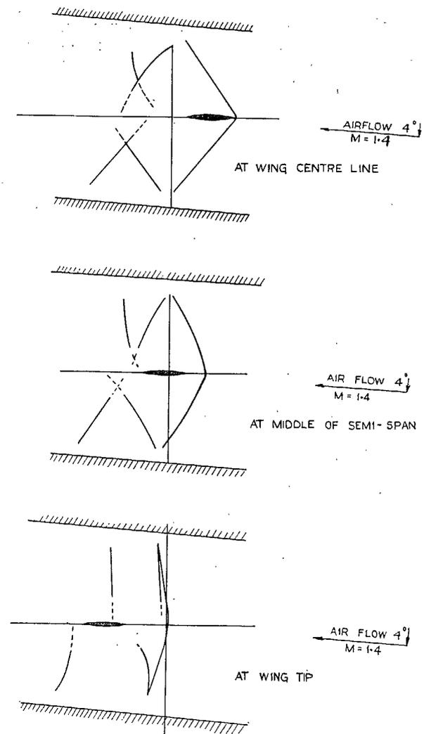
FIG. 6. Shock-wave configuration about a 50 deg swept-back wing,  $M = 1.4$ . Incidence = 4 deg. Sections in line of flight, perpendicular to the plane of the wing.
