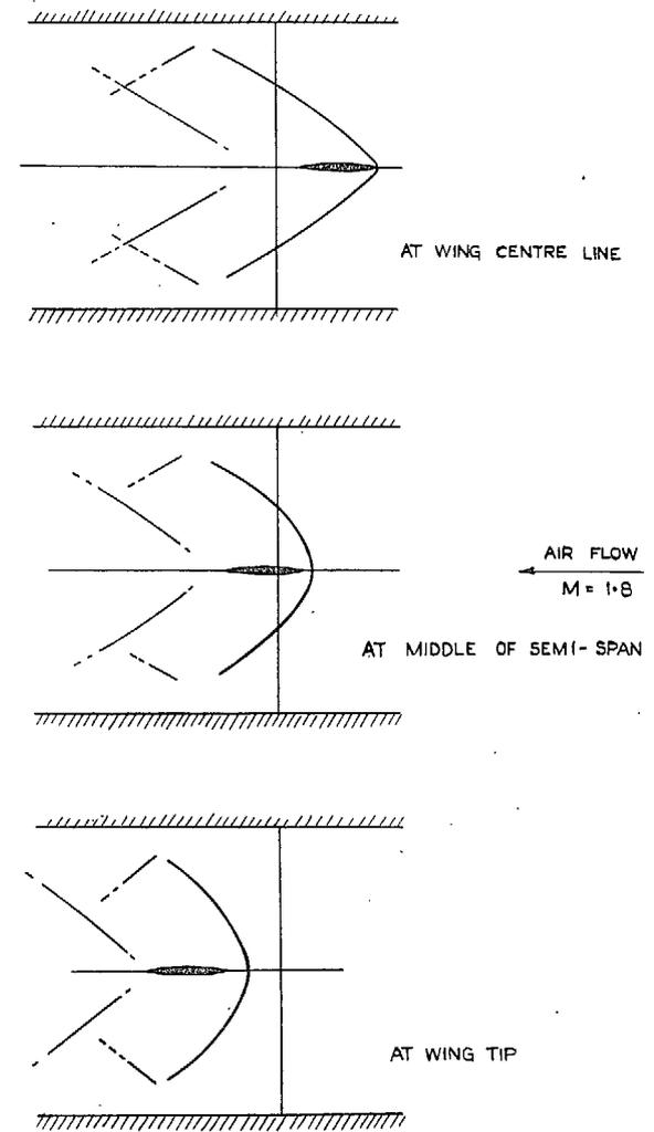
FIG. 10. Shock-wave configuration about a 50 deg swept-back wing,  $M = 1.8$ . Incidence = 0 deg. Sections in line of flight, perpendicular to the plane of the wing.
