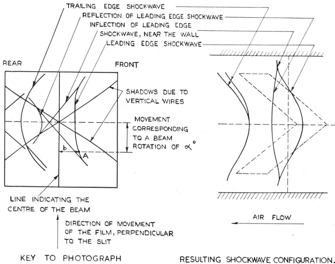
FIG. 4. Typical shock-wave photograph, with key.
