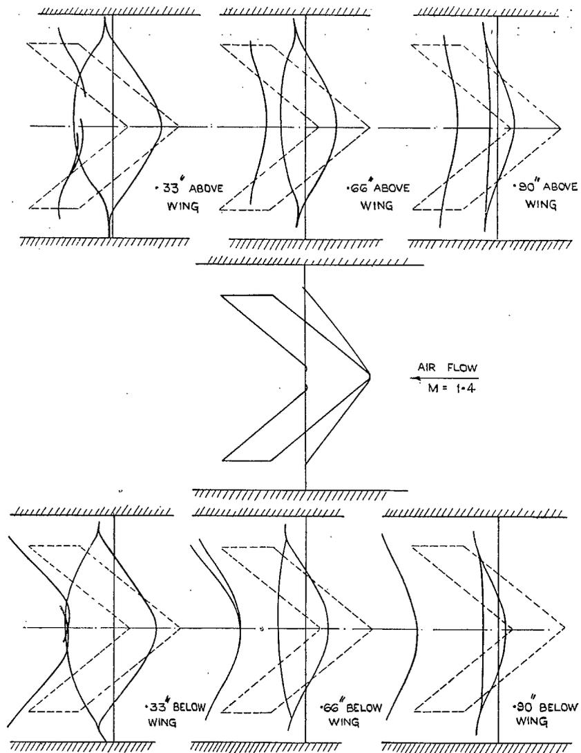
FIG. 5. Shock-wave configuration about a 50 deg swept-back wing,  $M = 1.4$ . Incidence = 4 deg. Sections parallel to the plane of the wing.
