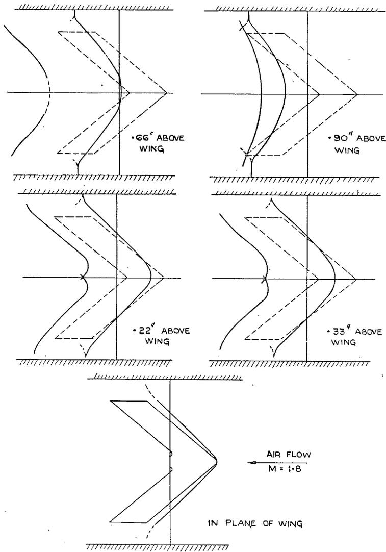
FIG. 9. Shock-wave configuration about a 50 deg swept-back wing,  $M = 1.8$ . Incidence = 0 deg. Sections parallel to the plane of the wing.
