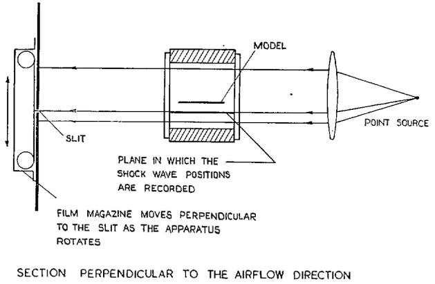
SECTION PERPENDICULAR TO THE AIRFLOW DIRECTION
