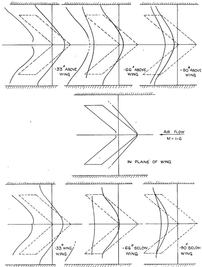
FIG. 7. Shock-wave configuration about a 50 deg swept-back wing,  $M = 1.6$ . Incidence = 4 deg. Sections parallel to the plane of the wing.
