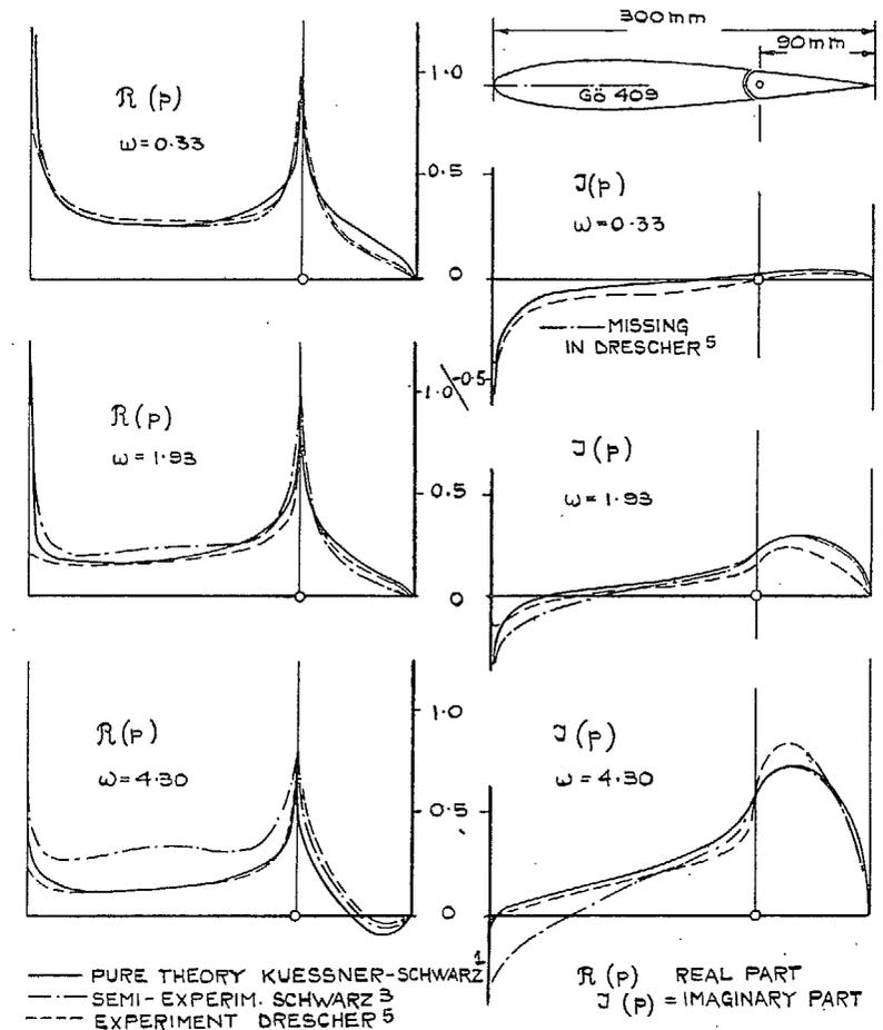
FIG. 6. Theoretical and experimental pressure distributions  $p(x, t)$  (Drescher).
