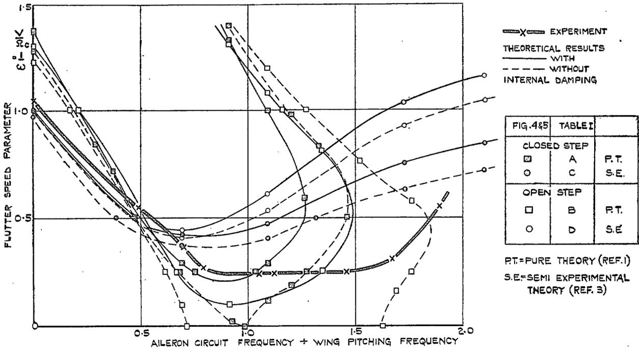
FIG. 4. Variation of flutter speed parameter with aileron circuit frequency.
