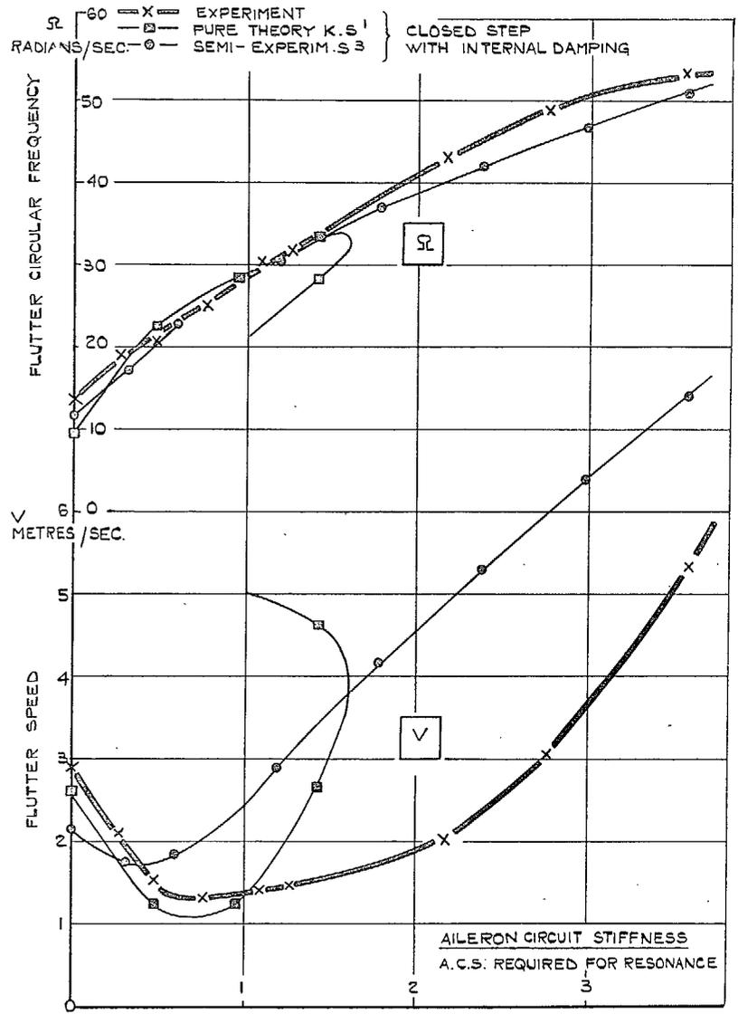
FIG. 5. Variation of flutter speed and frequency with aileron circuit stiffness.
