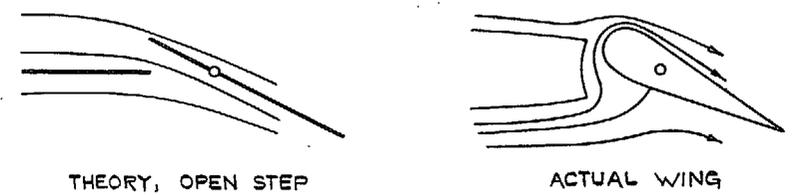
FIG. 7. Flow through wing aileron gap (diagrammatic).
