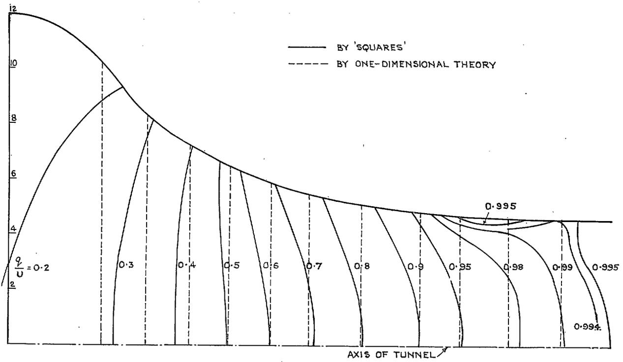
FIG. 2. Flow through a contraction in a circular tunnel—incompressible case.
