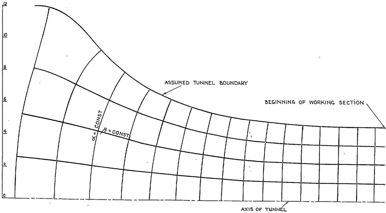
FIG. 1. Two dimensional network of stream and equipotential lines used as grid for the case of axial symmetry.
