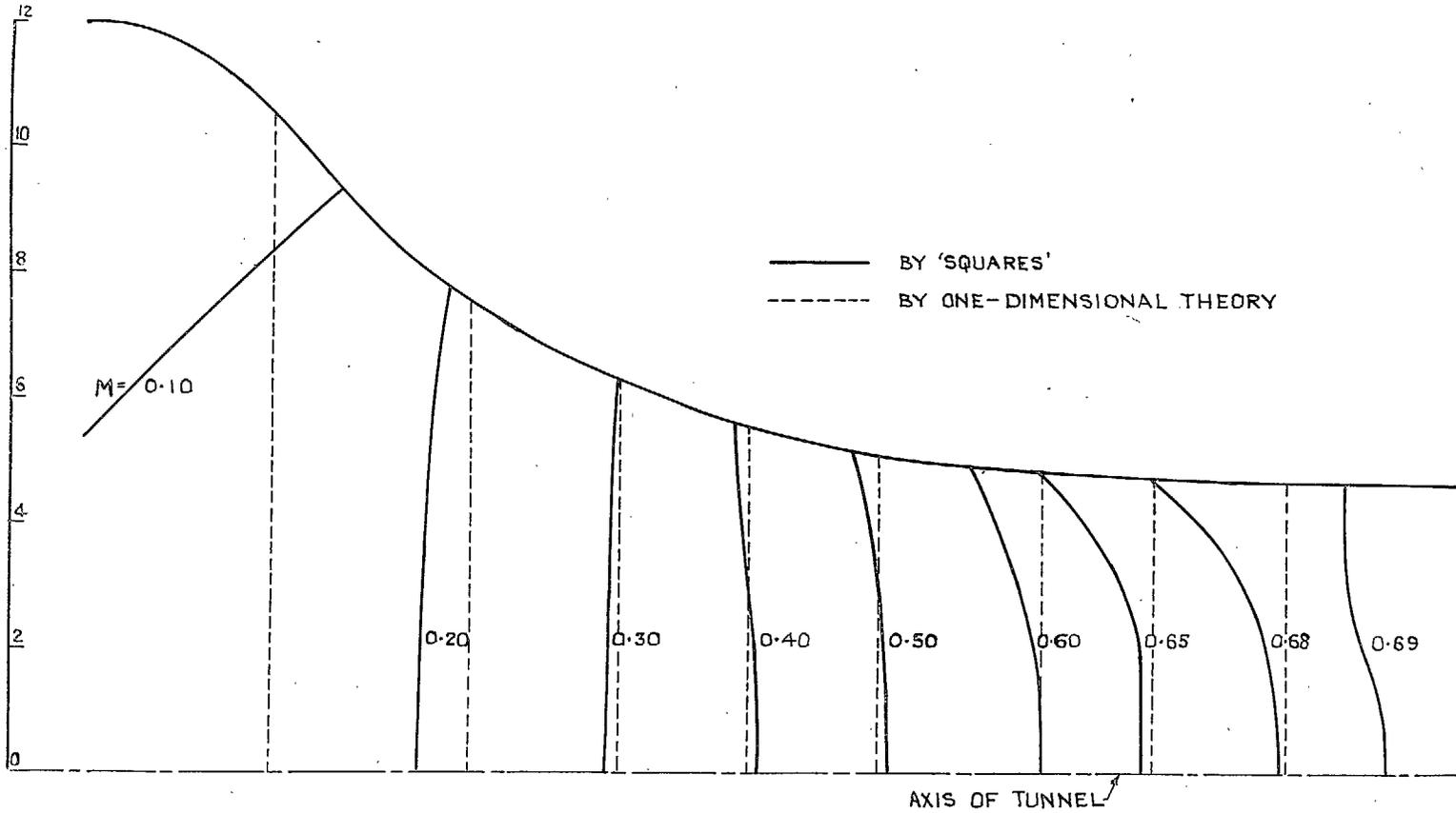
FIG. 3. Flow through a contraction in a circular tunnel—compressible case.
