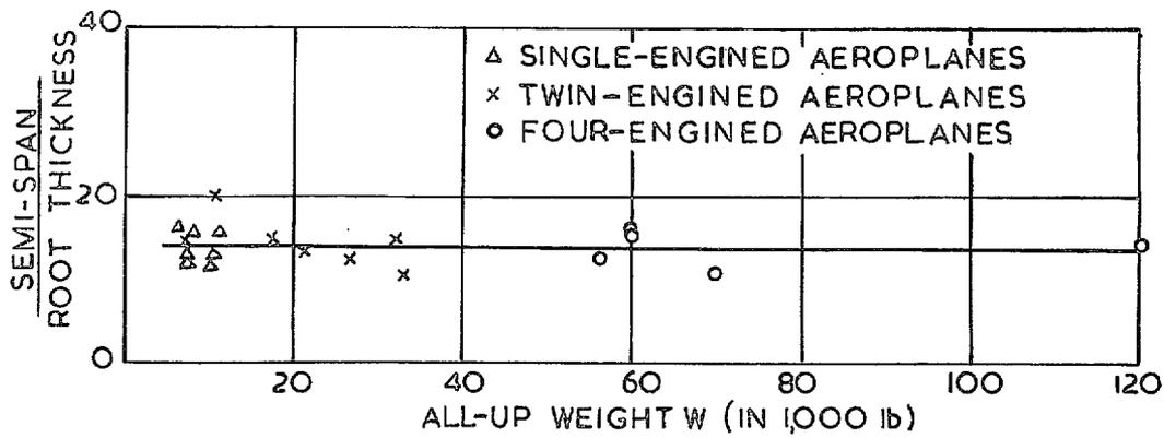
FIG. 1. Variation in Ratio of Wing Semi-span to Root Thickness with All-up Weight.
