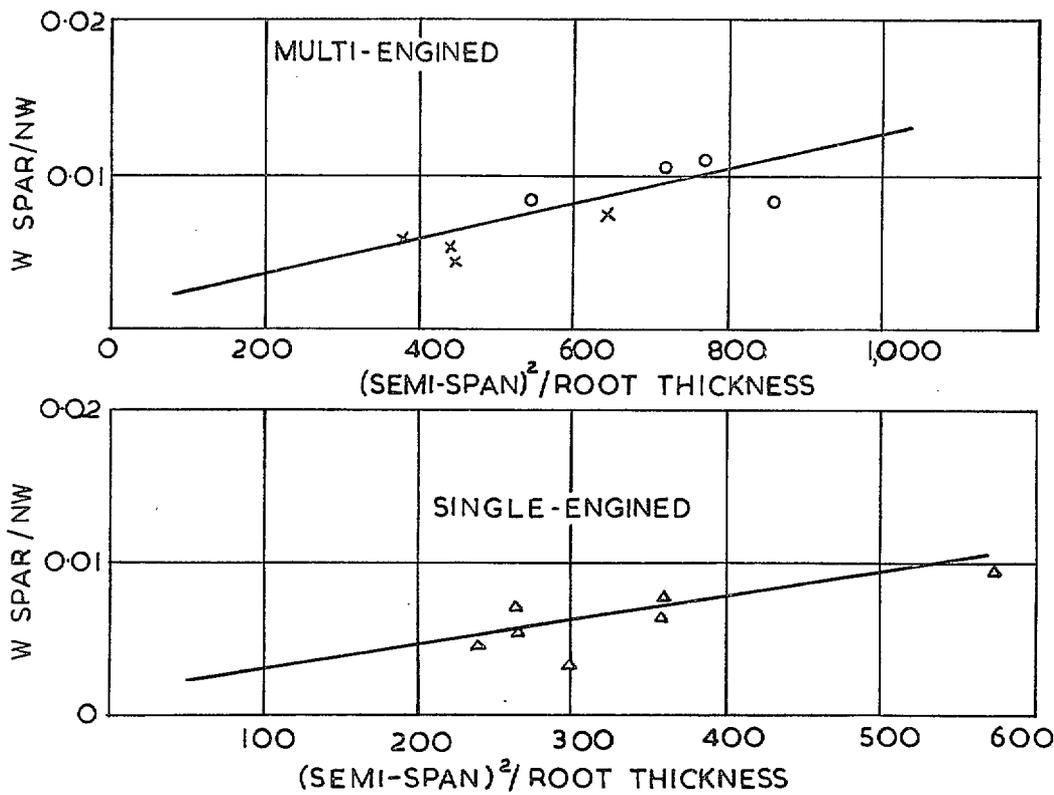
FIG. 2. Spar Weight Variation with Semi-span, Root Thickness, All-up Weight and Factor.
