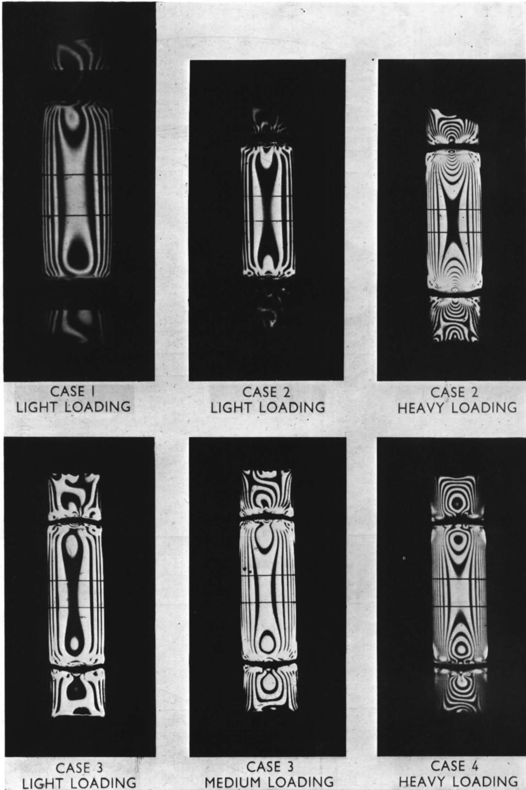
Photo-elastic model of cylindrical strut (for 1000-ton testing machine)
