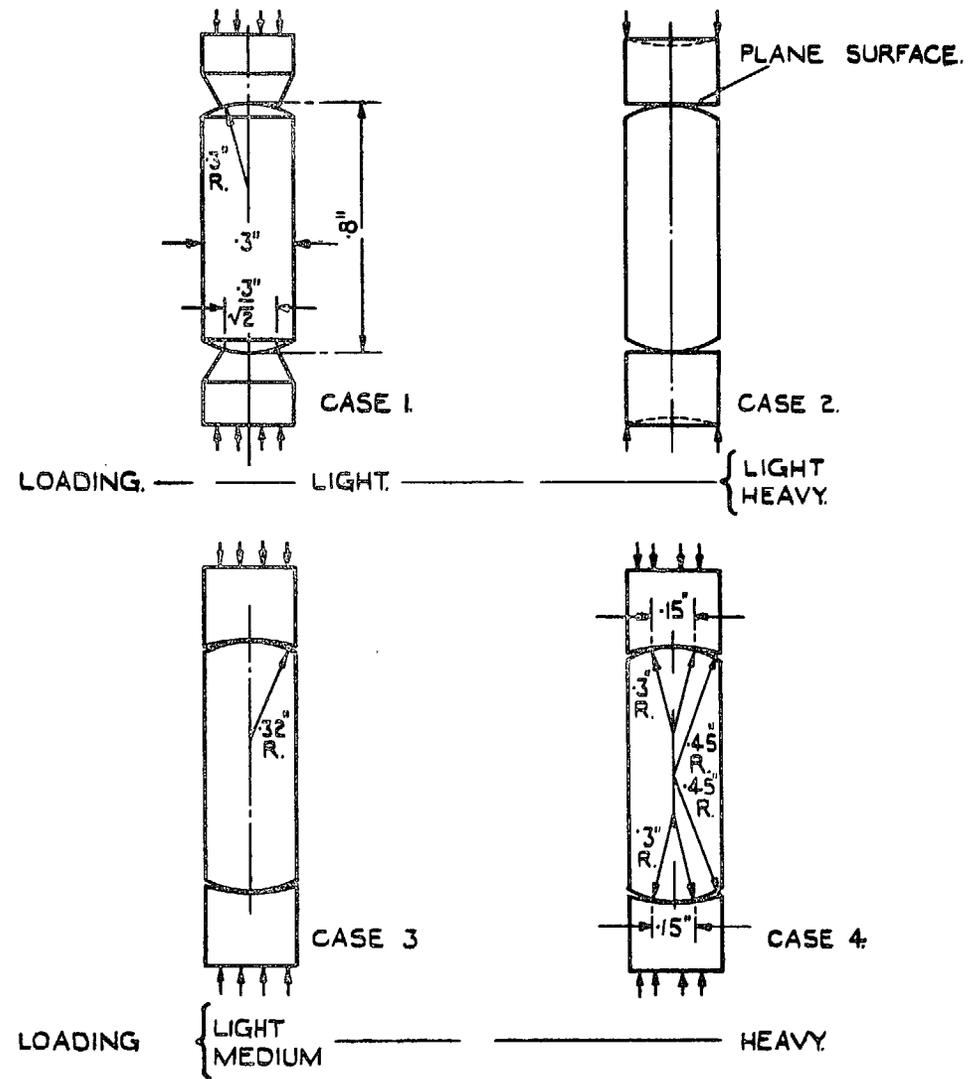
FIG. 2. Shapes of seating tested.
