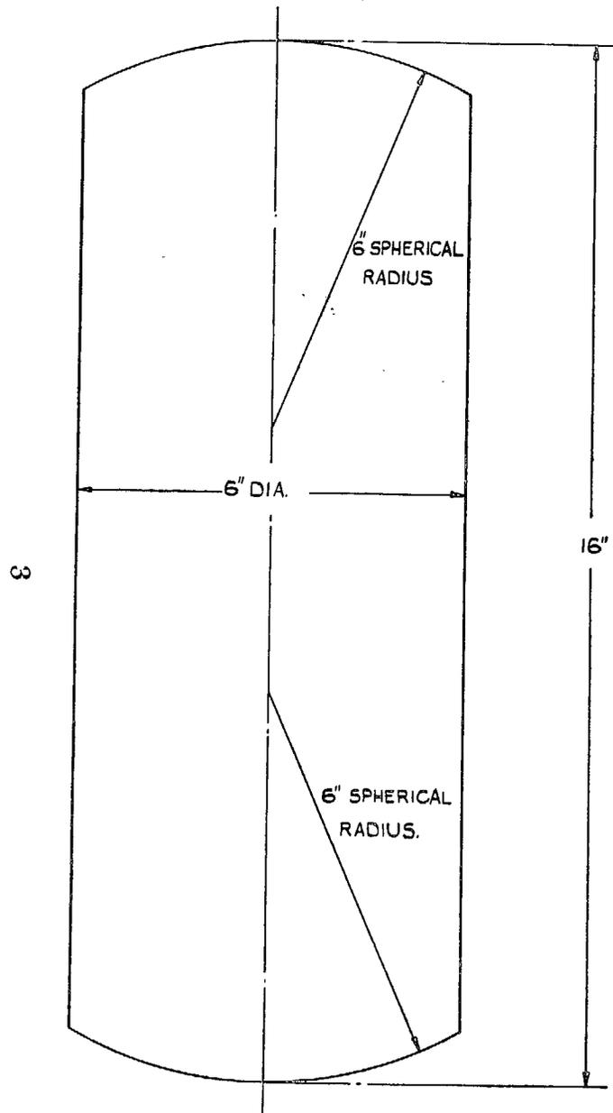
FIG. 1. Dimensions of steel strut.
