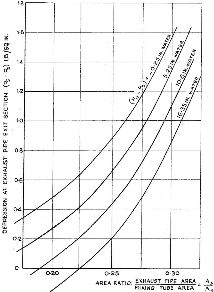
FIG. 4. Depression at Exhaust Outlet for Points Plotted in Fig. 2.
