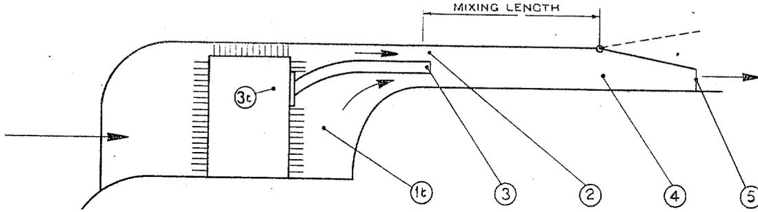
FIG. 1. Diagrammatic Sketch of Mixed Engine Exhaust and Cooling Air Systems.
