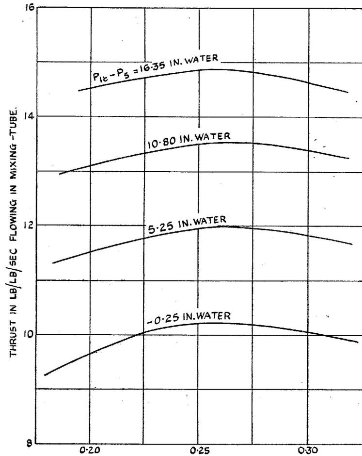
$$\text{AREA RATIO} = \frac{\text{EXHAUST PIPE AREA} - A_3}{\text{MIXING-TUBE AREA} - A_4}$$
