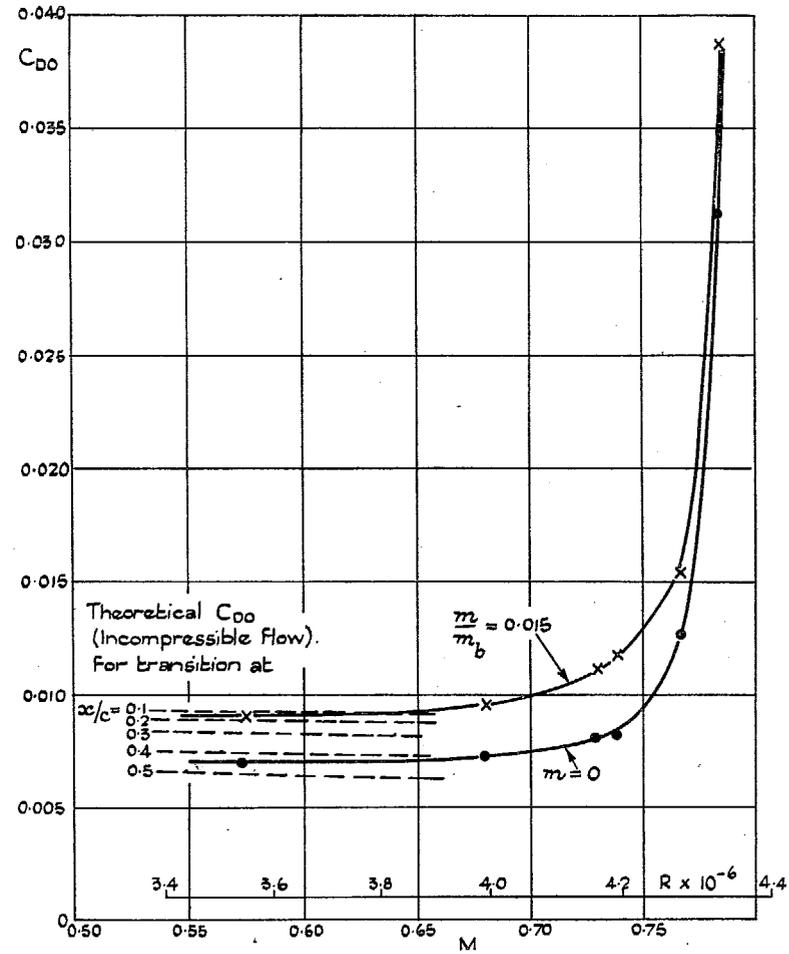
FIG. 5. Aerofoil EC 1250. 0 deg. Incidence.
