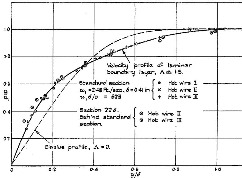
FIG. 2. Velocity Distribution in Boundary Layer on Floor.
