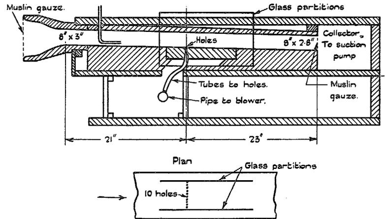
FIG. 1. Elevation View of Smoke Tunnel.
