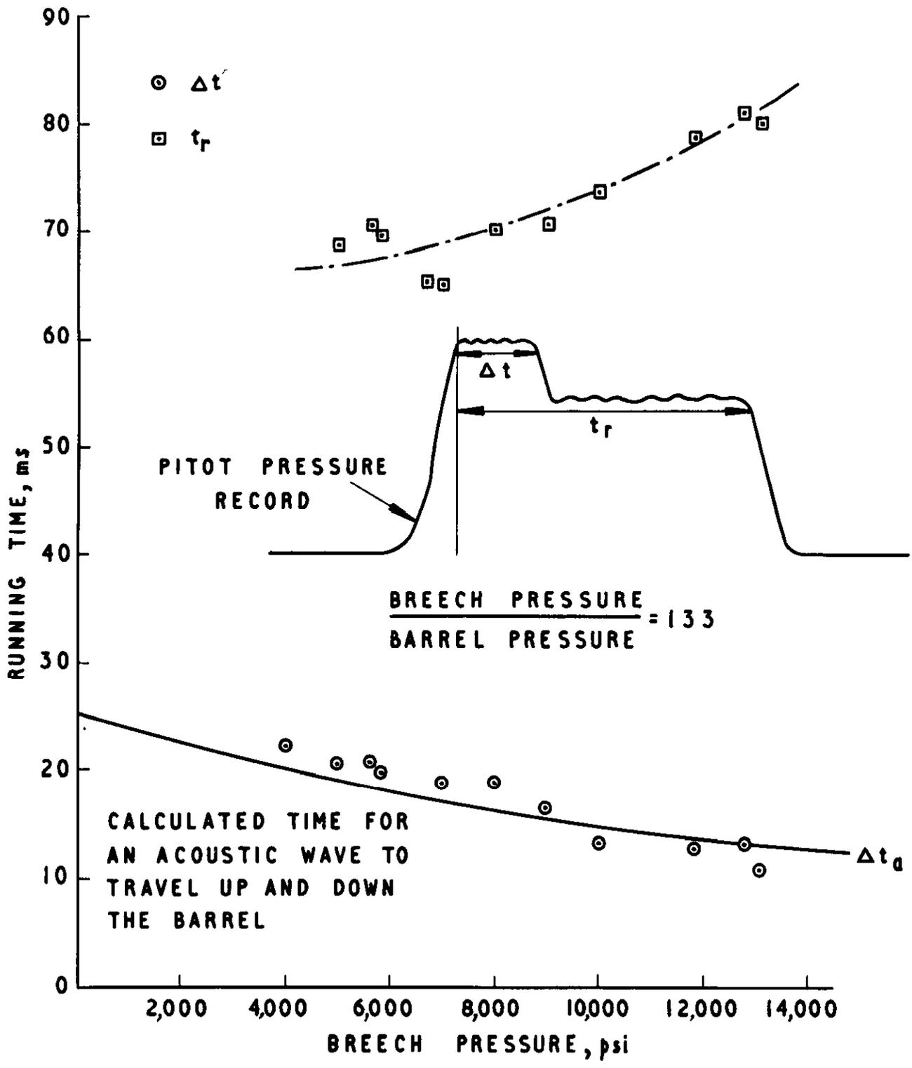
FIG. 4 RUNNING TIME AS A FUNCTION OF BREECH PRESSURE
