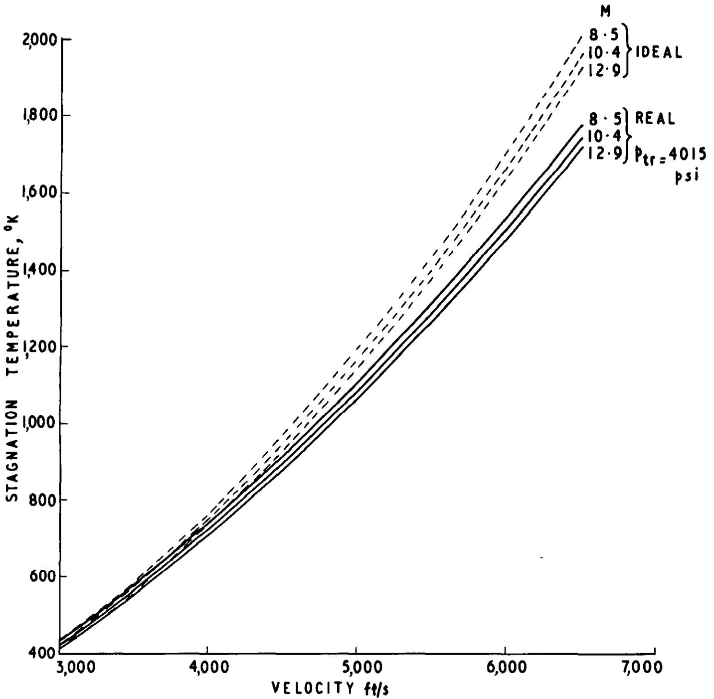
FIG I STAGNATION TEMPERATURE AS A FUNCTION OF FLOW VELOCITY
