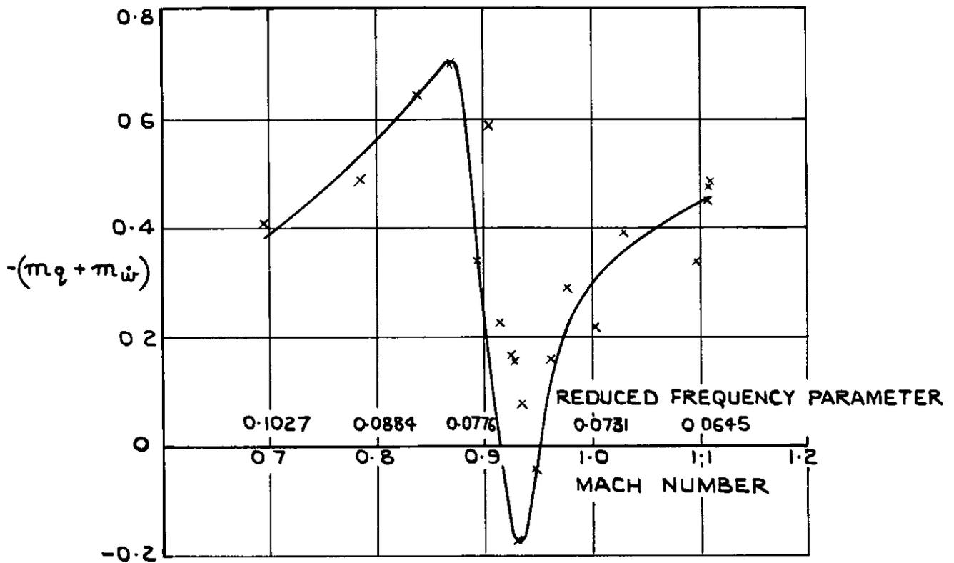
(a) VARIATION OF  $-(m_q + m\dot{\omega})$  WITH MACH NUMBER. CONFIGURATION A-WING BODY COMBINATION.
