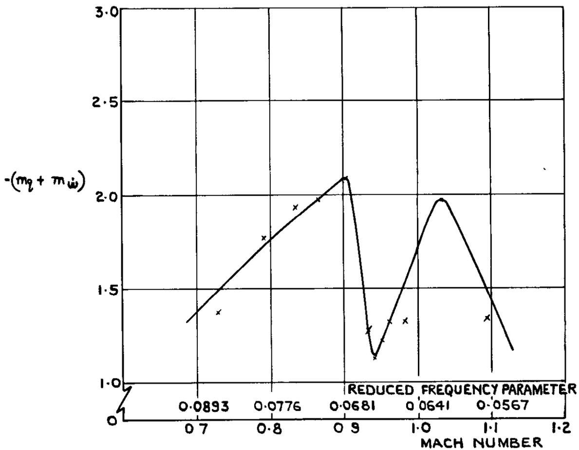
(a) VARIATION OF  $-(m\ddot{q} + m\dot{\omega})$  WITH MACH NUMBER. CONFIGURATION C WING BODY + TAIL (LONG ARM.)
