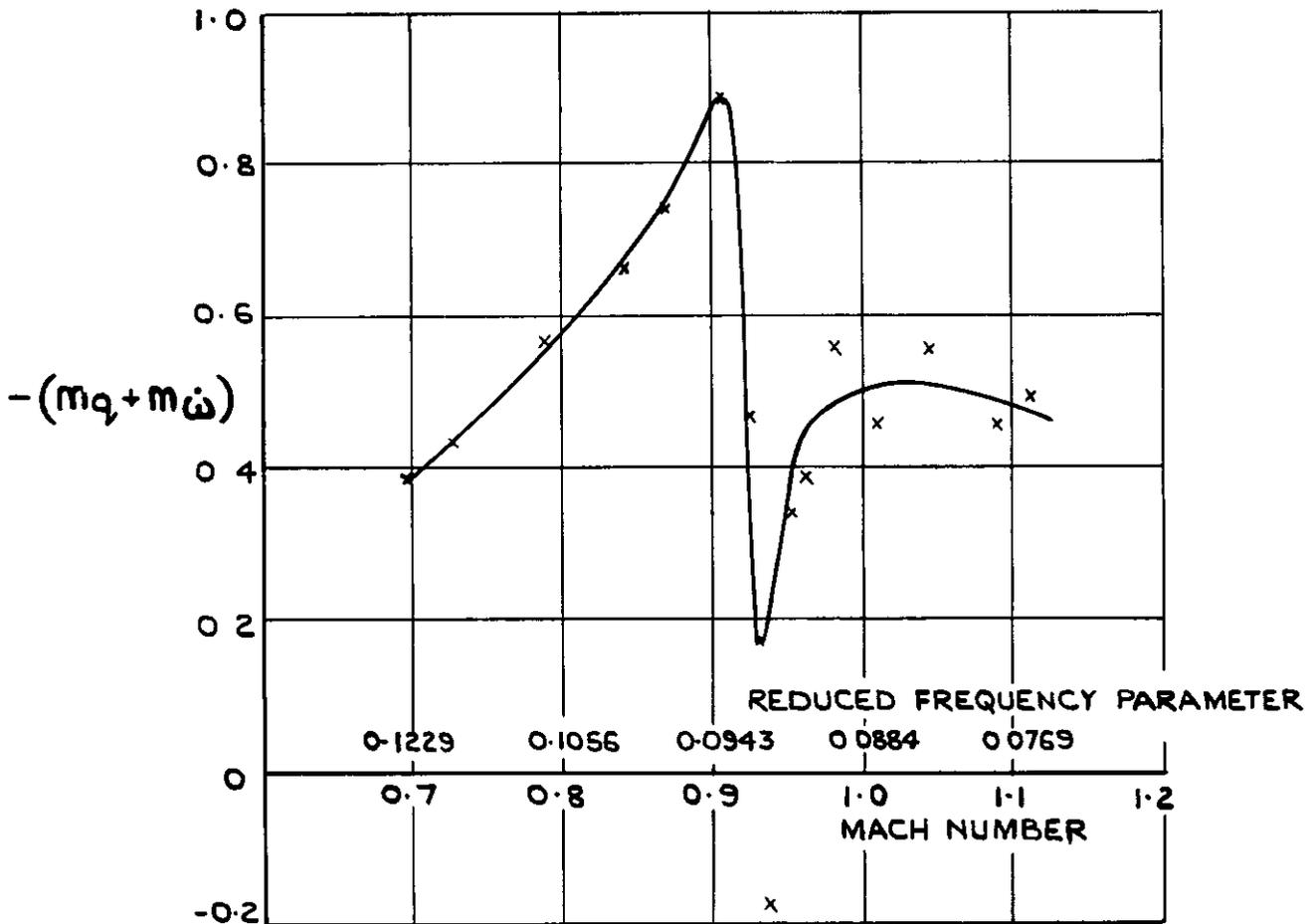
(b). VARIATION OF  $-(m_q + m\dot{\omega})$  WITH MACH NUMBER. CONFIGURATION A - WING BODY COMBINATION.
