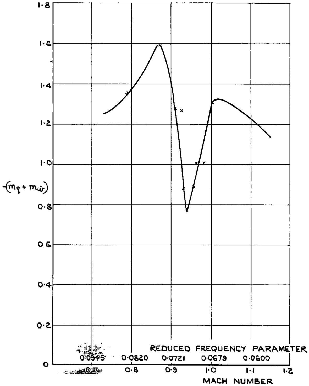
**FIG. 3. VARIATION OF  $-(m_q + m_{\dot{w}})$  WITH MACH NUMBER. CONFIGURATION B- WING BODY + TAIL (SHORT ARM.)**
