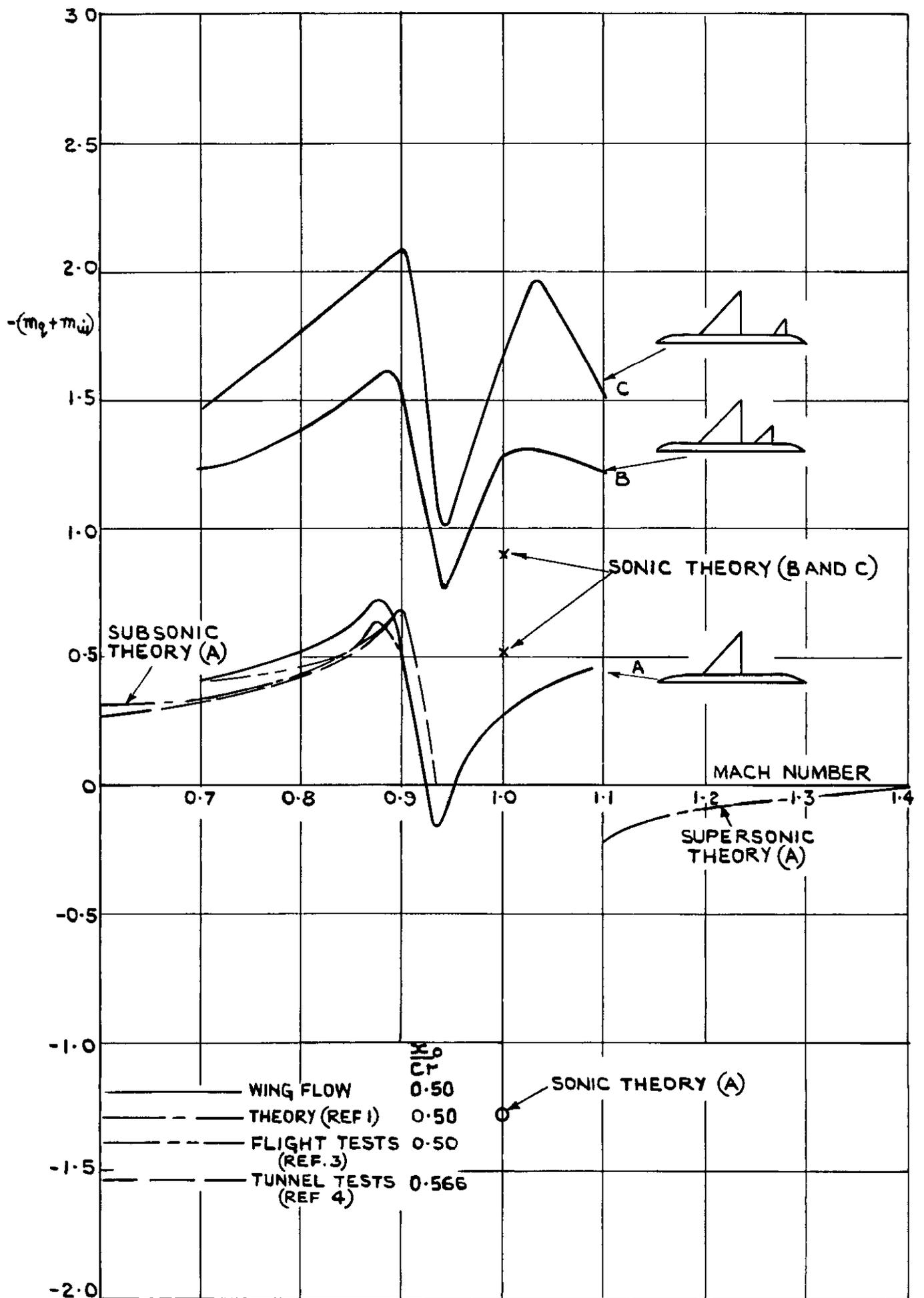
FIG. 5. COMPARISON OF  $-(m_q + m_w)$  FOR THE THREE CONFIGURATIONS, A, B AND C.
