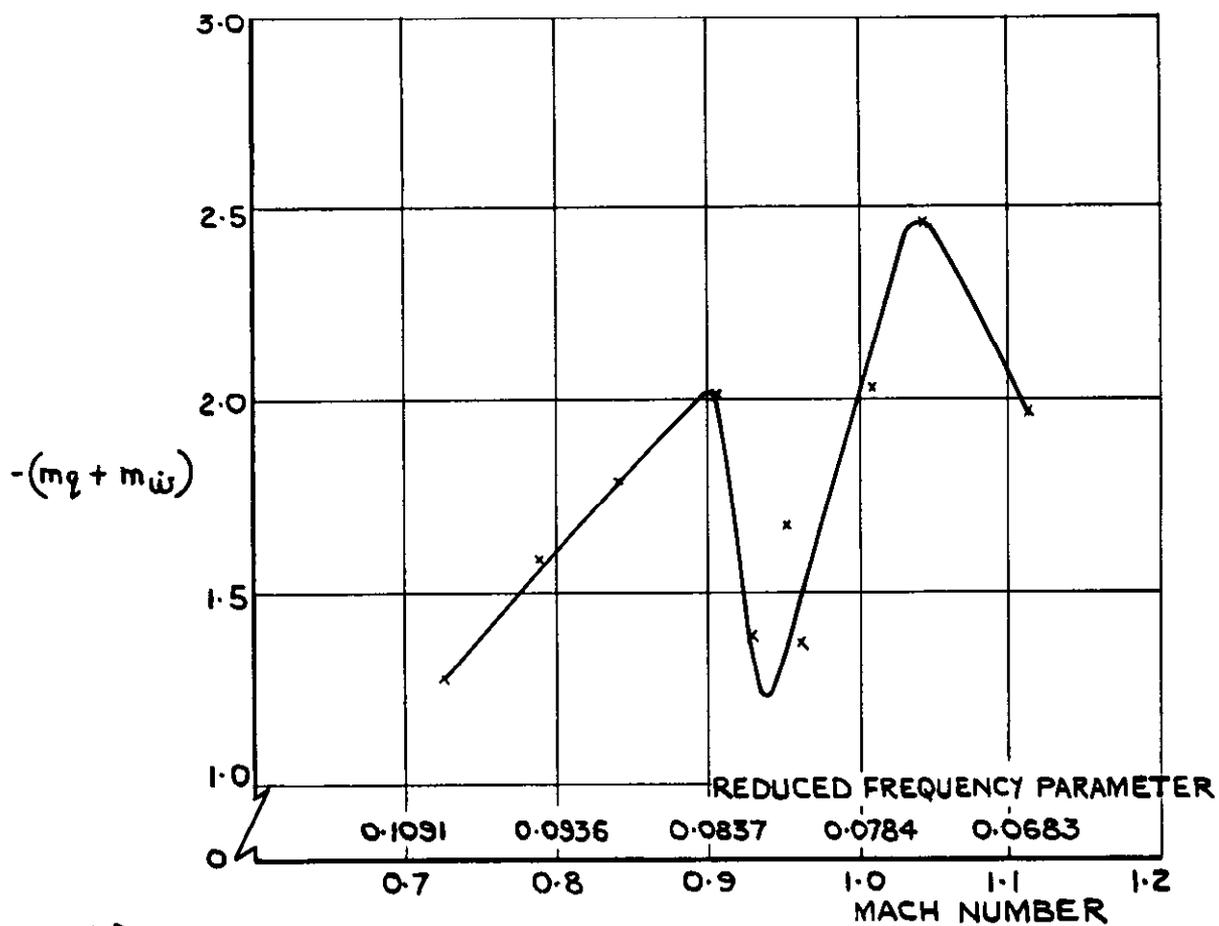
(b) VARIATION OF  $-(m\ddot{q} + m\dot{\omega})$  WITH MACH NUMBER. CONFIGURATION C WING BODY + TAIL (LONG ARM.)
