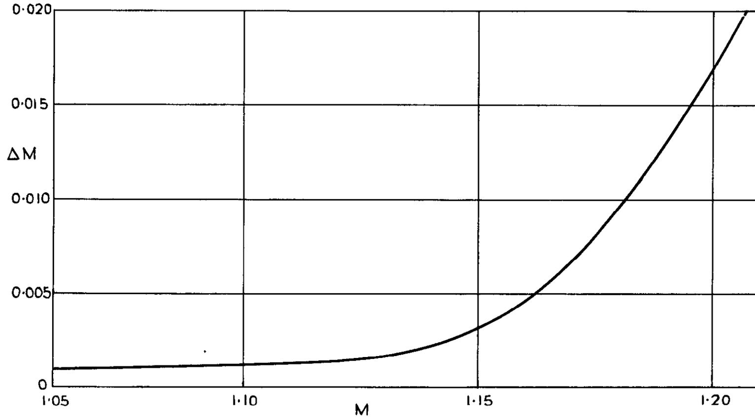
Correction to the indicated Mach number due to the pressure gradient between the reference hole and the model position
