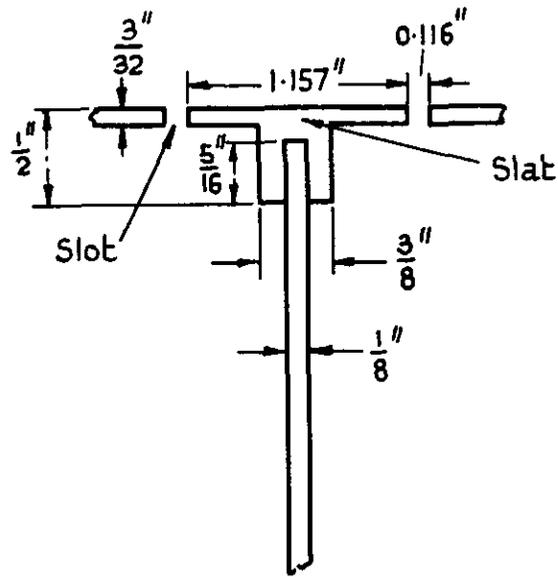
The detail design of a slat. Cross-section taken perpendicular to the tunnel axis at AA' (see fig 1)
