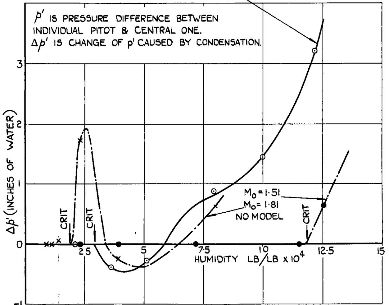
**FIG.8(a&b) VARIATION OF PITOT PRESSURE WITH HUMIDITY WITH & WITHOUT MODEL.**
