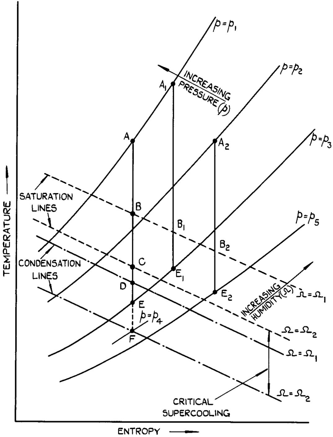
FIG.2. ISENTROPIC EXPANSION OF WATER VAPOUR ON THE TEMPERATURE - ENTROPY DIAGRAM.
