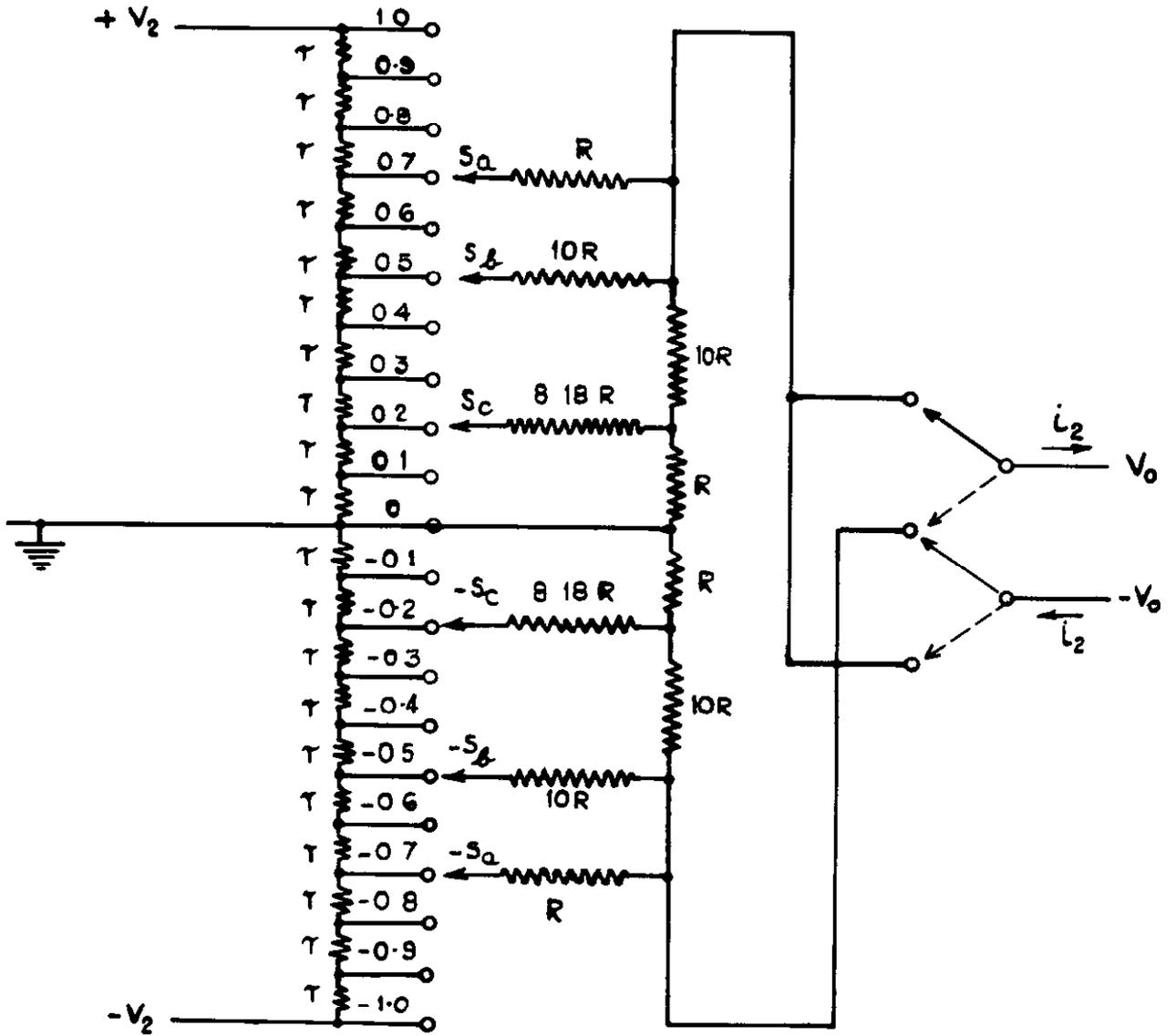
FIG.5. POTENTIOMETER AND REVERSING UNIT
