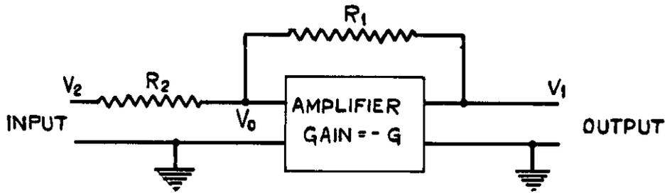
FIG. 1 AMPLIFIER WITH RESISTANCE FEEDBACK.
