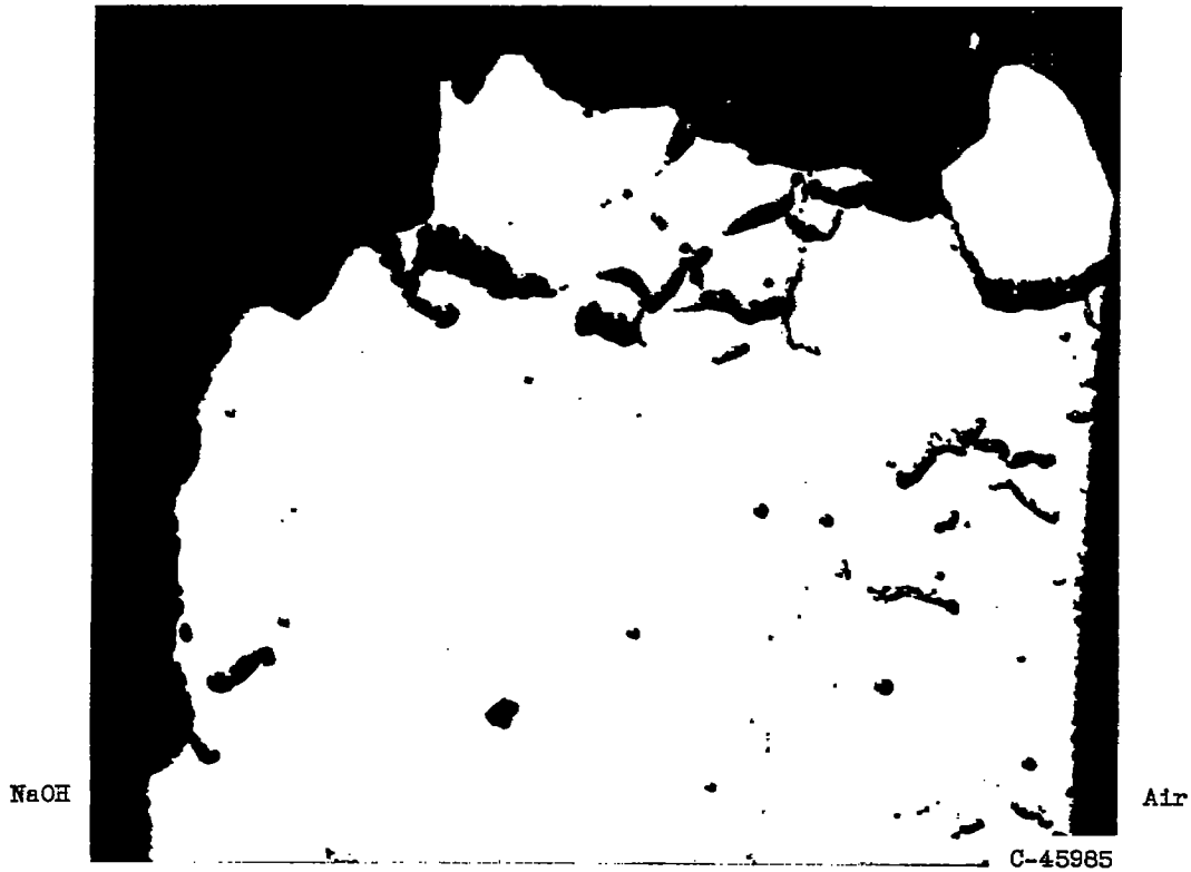
Figure 11. - Fracture of tube that contained NaOH and was tested in air at 1500 psi and 1500° F for 592 hours. Unetched. X75.
