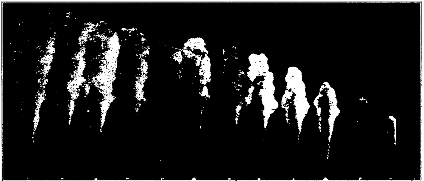
FIG. 8.—Injection pressure, 8,000 lb./sq. in. Chamber pressure, 300 lb./sq. in. The original photographs for figures 3 to 8 inclusive were retouched for reproduction purposes
