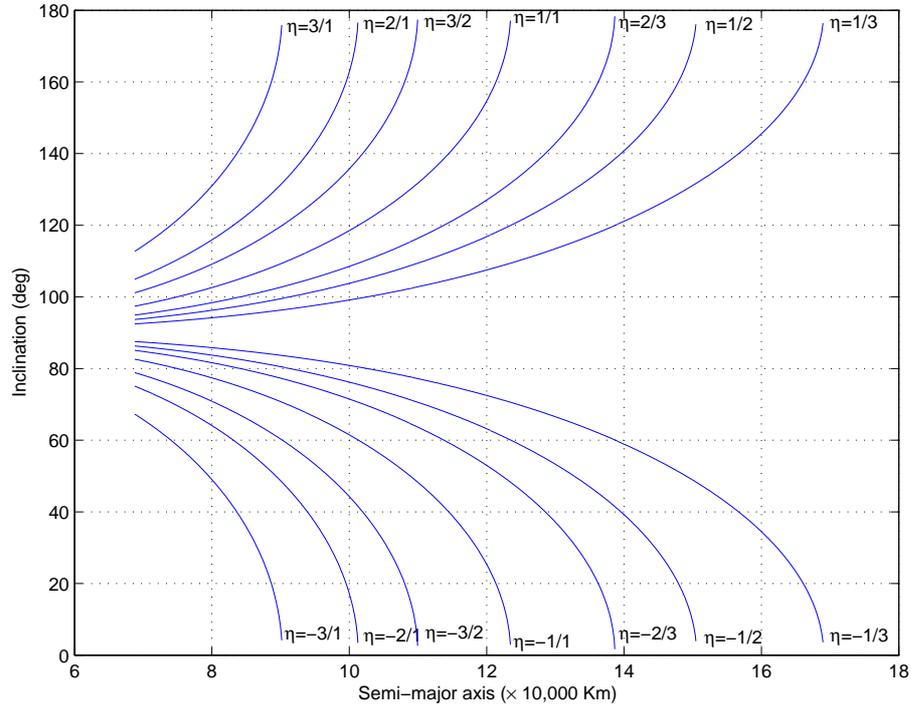
Figure 5: Multi Sun-Synchronous Circular Orbits: Type II
