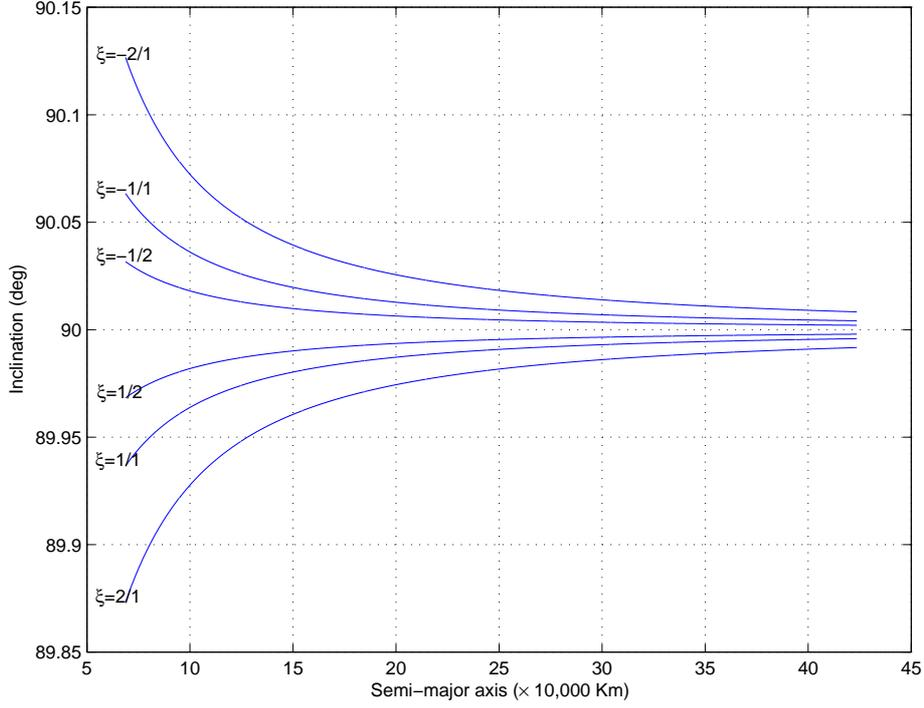
Figure 4: Multi Sun-Synchronous Circular Orbits: Type I
